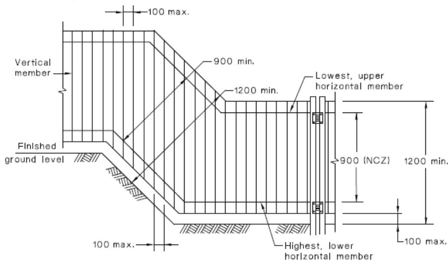
NOTE: On sloping sites, the fence height is to be measured perpendicular to the ground line.
