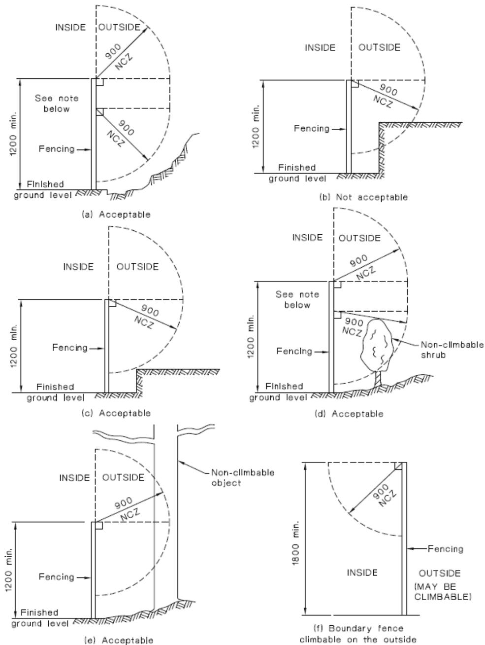
NOTE: The lower radius point may be anywhere on the fence at least 900 mm above the ground or the highest lower rail or foothold.
